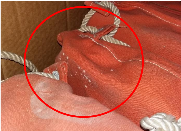
Figure 12: Mould growing on life jackets (textile) in the store. Photo by author
